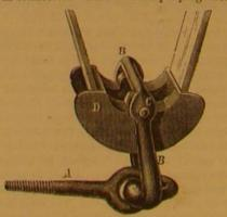
The part, A, screws into the end of the neck yoke, in the usual manner. The ring, B, is made of an elongated angular shape, as shown, and has pivoted to it, at C, a slide, D. This slide is made with a broad surface, upon which the breast strap draws; the method of pivoting allowing any ordinary motion of the ring to take place without any sliding of the strap on the ring and consequent wear. The strap is, moreover, kept smooth and flat on the slide, which also adds to its durability.
