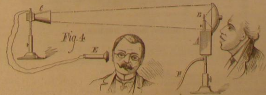
THERMOPHONE WITH THERMO-ELECTRIC RECEIVER AND MANOMETRIC FLAME TRANSMITTER.
