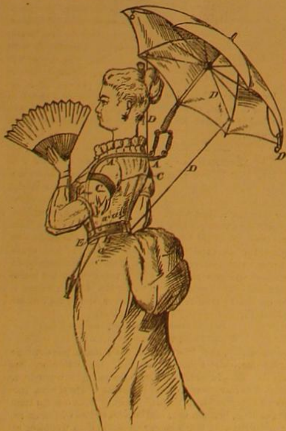
A A are two rods, curved to fit upon the forward side of and pass over the shoulders of the wearer. The lower ends of the rods, A A, are attached or hinged, as shown at a', to an
