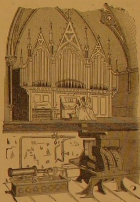
Lascell's Organ-Blowing Apparatus (Dr. Partridge's Church, Brooklyn, N. Y.).
